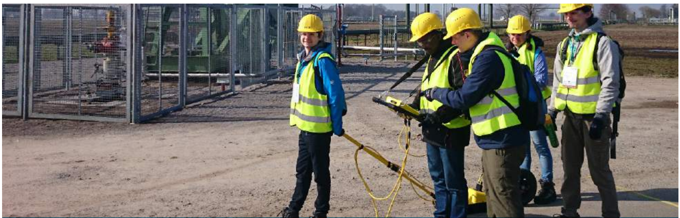
Figure A: Infrastructure survey with a pulseEKKO PRO 500 MHz system
