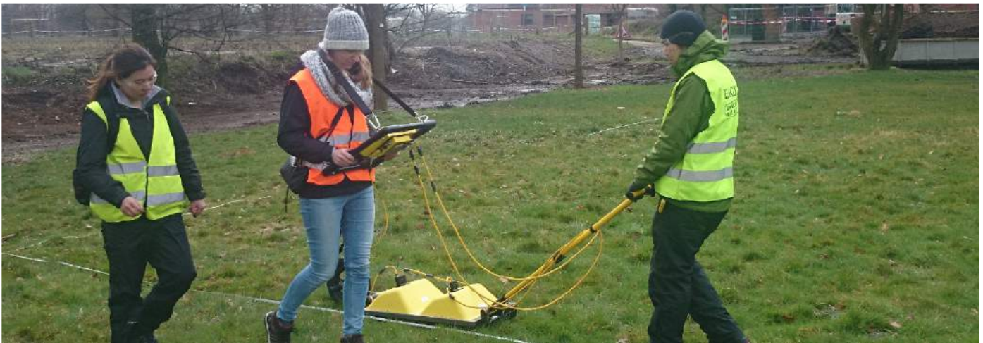
Figure C: Archaeological survey using 250 MHz transducers
