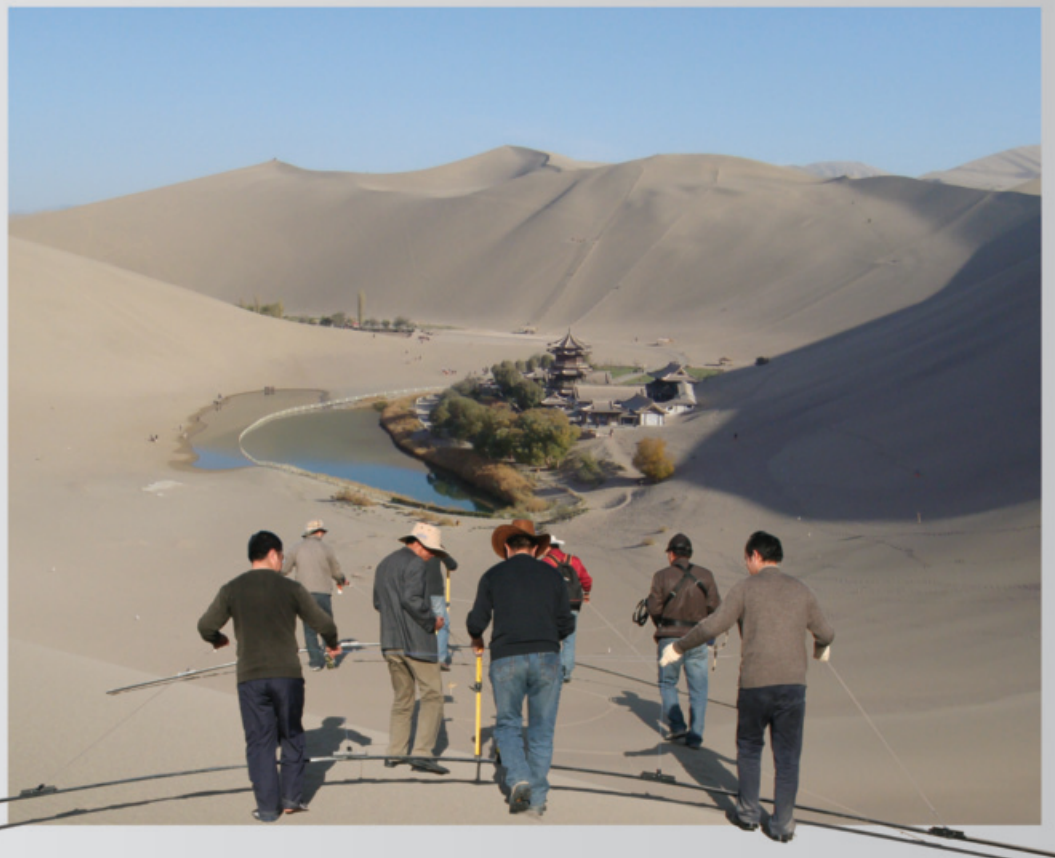
Figure 1: Survey team carrying 12.5 MHz antennas along the crest of the dune in north western China.
